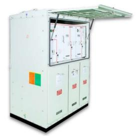
Ring Main Unit is a fully enclosed, compact, factory assembled cabinet used for medium-voltage power distribution. In simple words, this is a switchgear unit that is easily replaceable, requires low maintenance, and is highly protected in nature. The most common versions of RMU are Extensible & Non- extensible types - 3 Function & 4 Functions. A typical 3 function RMU shall comprise of 2 x 630 Amps Load Break Switch + 1 x 200/400/630 Amps Circuit Breaker (SF-6 or Vacuum type).
